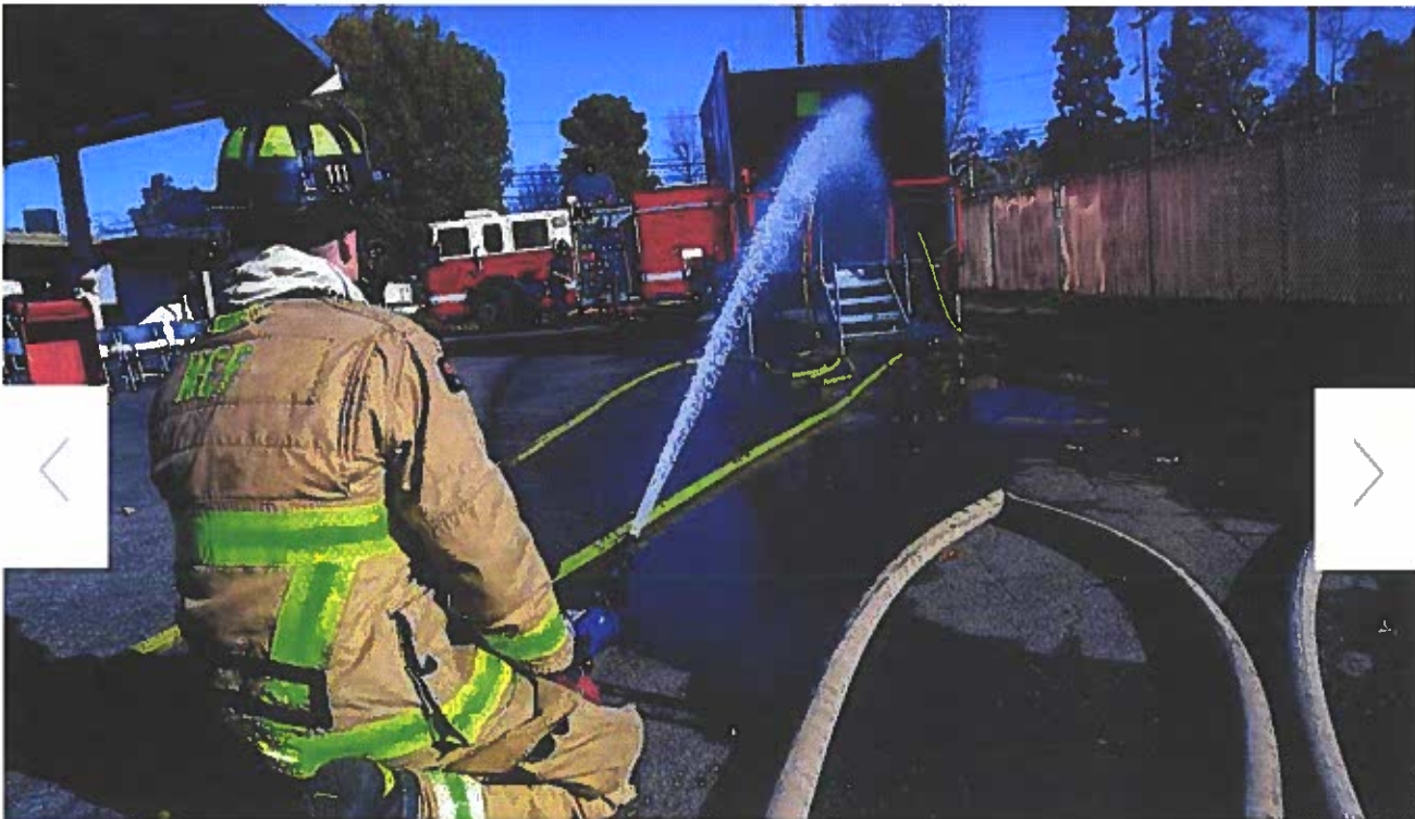
North County firefighter Max Paur sends water from a firehose into the Pump Pod. The Pump Pod allows firefighters to train in pump control valve operation without wasting water. The water
