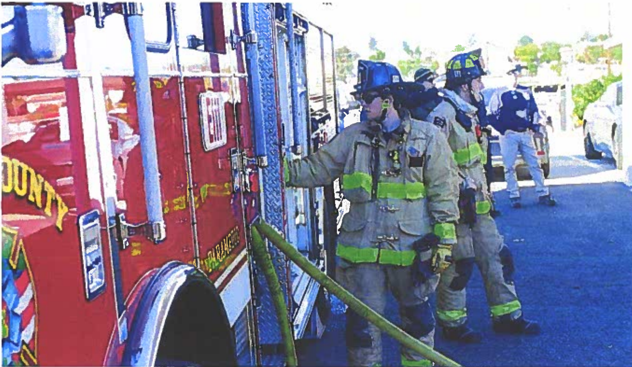
North County firefighter Kyle Krenz operates pump control valves on a fire engine during a demonstration of NCFPD's new water saving Pump Pod. Village News/Shane Gibson photo
